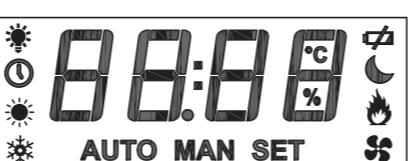
4-digit multifunction indicator for temperature display, reduced set point, clock and user / installer settings.
